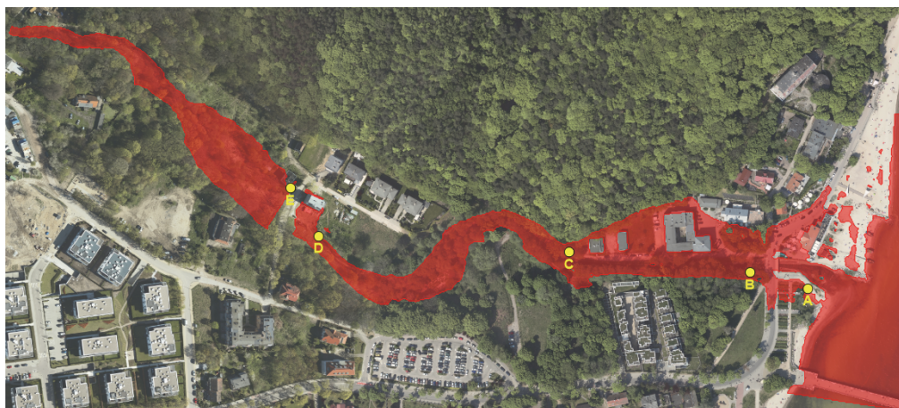
Fig. 7. Maximum range of flooded area along the whole analyzed section of Kacza river in variant 3 together with depicted measurement points (A, B, C, D, E) of maximum water level ordinates after the flood in July 2016 (image prepared by this author on the basis of orthophotomap from municipal geodesic resources of Gdynia, Gdynia Municipal Council licence No. PND.6642.1.1697.2018_2262_N, without scale)
