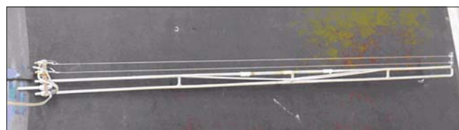
Fig. 10. Resistive wave gauge manufactured at CTO S.A.
