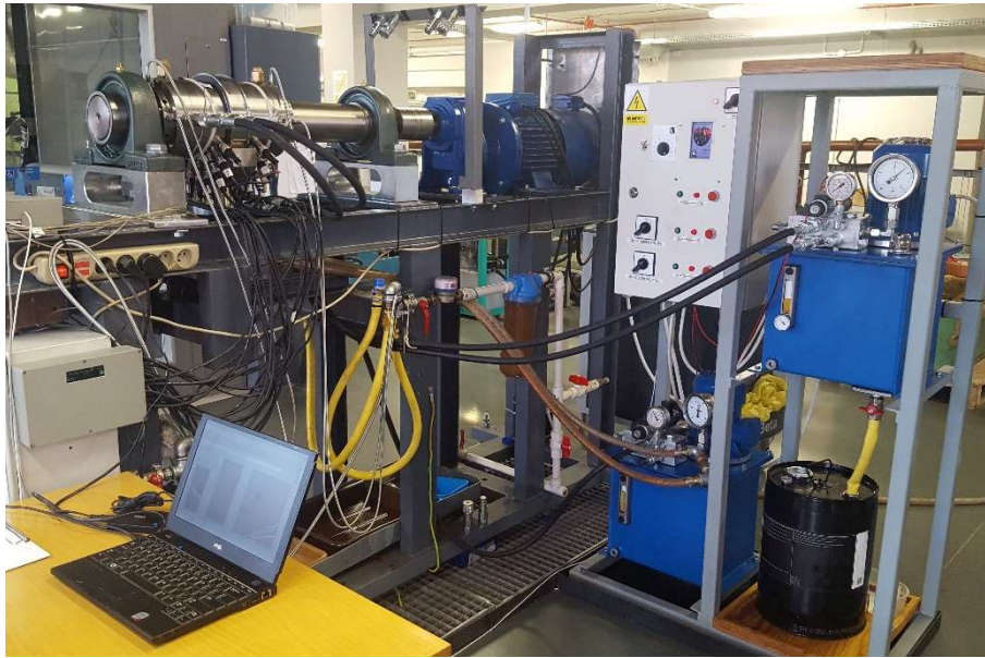
Figure 1. Test stand for marine stern tube bearings during tests of oil lubricated bearings
