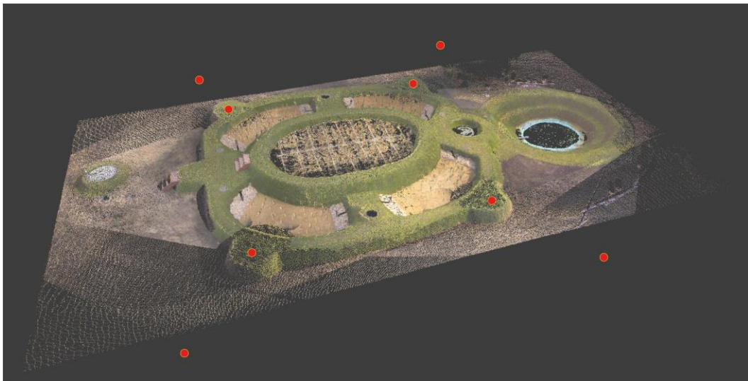
Fig. 3. Natural-colour visualisation of the combined point cloud with scanning locations (marked with red dots).
