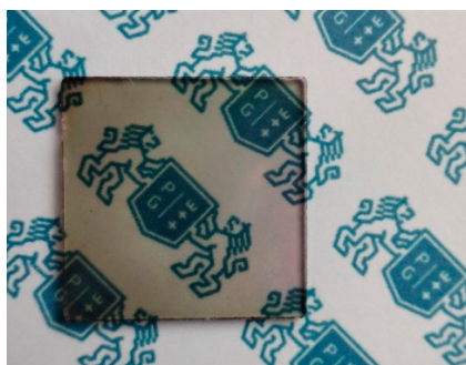
Figure 1. Picture of the fabricated sample: growth at 700 °C with a 2000 ppm [B]/[C] ratio.
