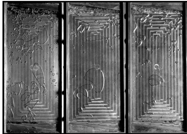
Figure 8. The intensity of the boiling process for three minigap thicknesses and for the same filling height (water): Left —1 mm, middle —2 mm, right —3 mm.
