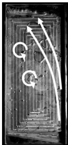
Figure 24. The way of flow distribution for an adiabatic flow of the water–air mixture.
