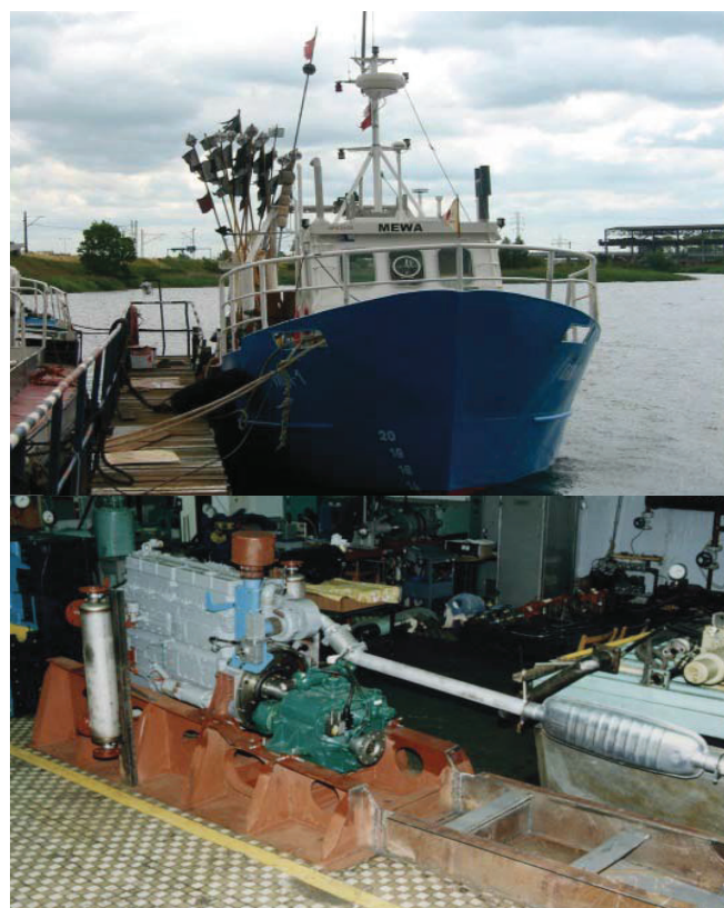
Fig. 3. KR-10 fishing vessel: propulsion system with hydraulic drive of technological devices [7]
