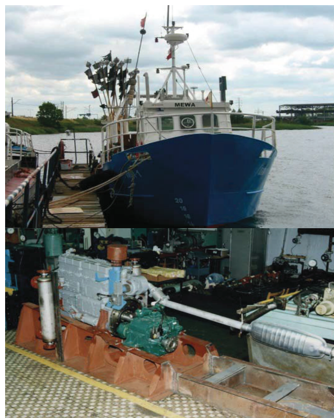
Fig. 3. KR-10 fishing vessel: propulsion system with hydraulic drive of technological devices [7]
