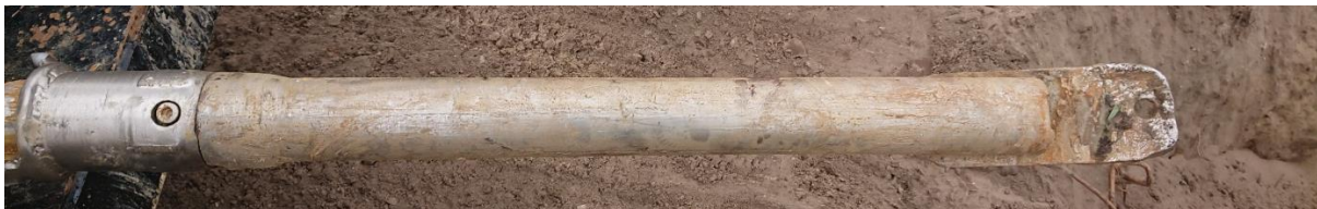
Figure 1. Pilot drill head
