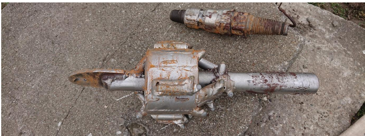
Figure 2. Reaming and flushing heads
