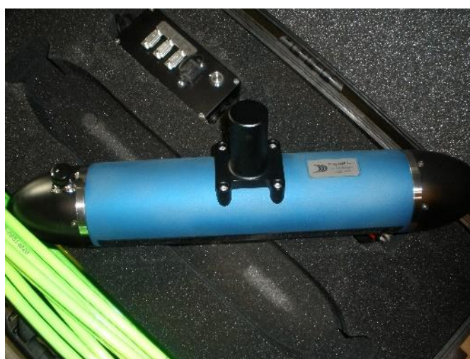
Figure 1. Photograph of the 3D Sidescan 3DSS-DX-450 sonar system (photograph: A. Stateczny).
