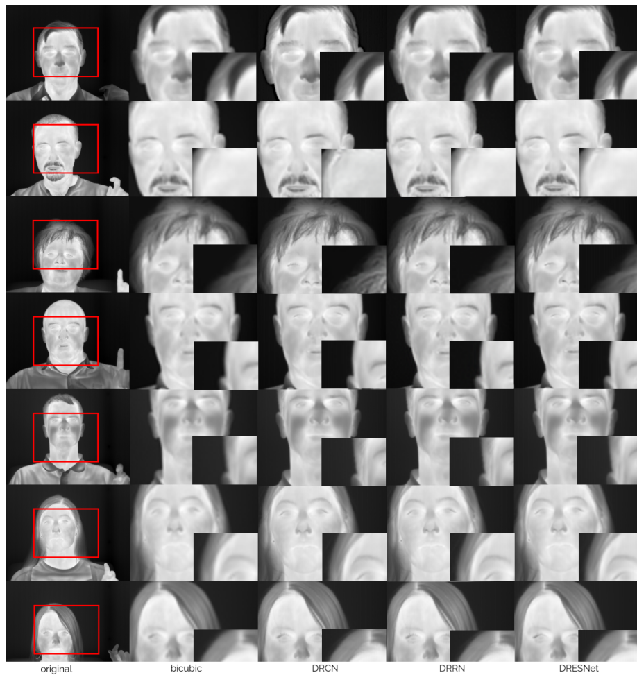
Figure 7: Thermal images after decreasing and increasing image resolution. From the left: original image with a marked facial area, the enlarged region of the marked facial area and enlarged chosen facial features in images after applying bicubic interpolation, DRCN, DRRN and the proposed DRESNet model.
