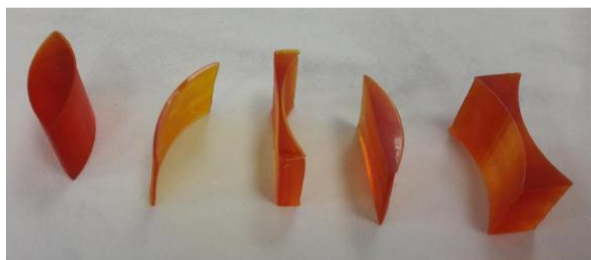
Fig. 1. Prototypes of cylindrical lenses which were printed using a 3D printer. From the left: convexo-convex lens, convexo-concave lens, plano-concave lens, plano-convex lens, concavo-concave lens.
