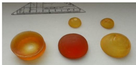
Fig. 2. Prototypes of printed spherical lenses. From the bottom left: plano-concave lens, plano-convex lens, and convex-concave lens. In the upper part of the photo, there are two convex-concave lenses.
