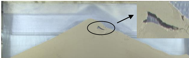
Fig. 2. Shape of the macropore corresponding to its maximum volume, t=1200s .
