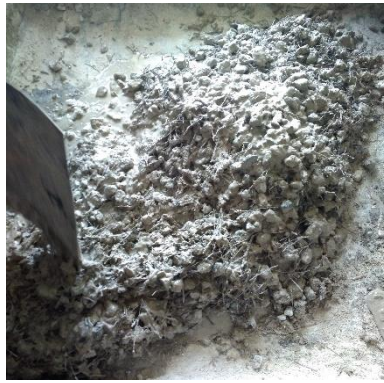
Fig. 1 Mixing of the HFRGC
