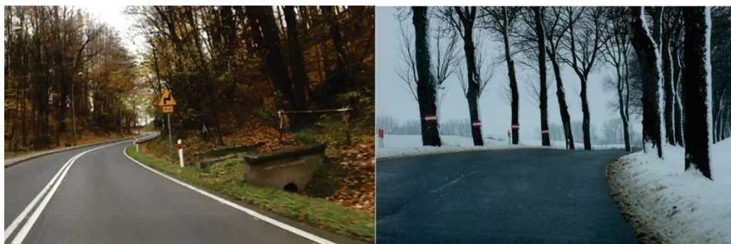
Fig. 1 Examples of roadside hazards on horizontal curves.
