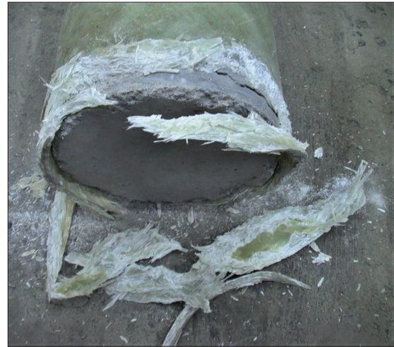
Fig. 2. Destruction (debonding) of a pipe made of glass fibre reinforced composite
