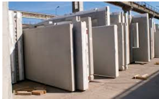
Figure 2. Prefabricated elements storage.
