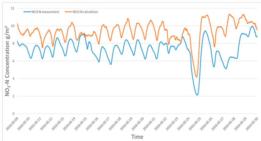
Figure 4. The comparison between the measured versus calculated “virtual” NO 3 -N data by model predictions at the “Klimzowiec” WWTP.
