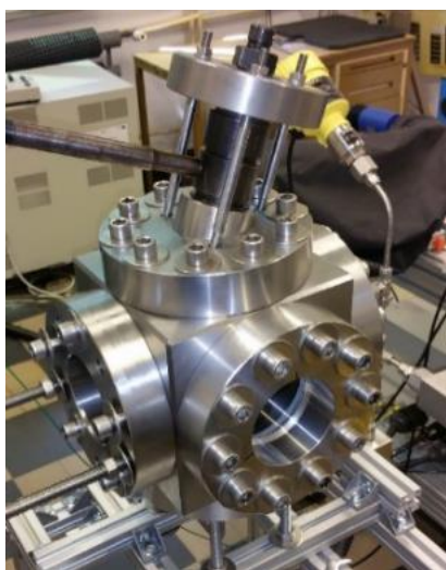
Fig. 1 Constant volume chamber
