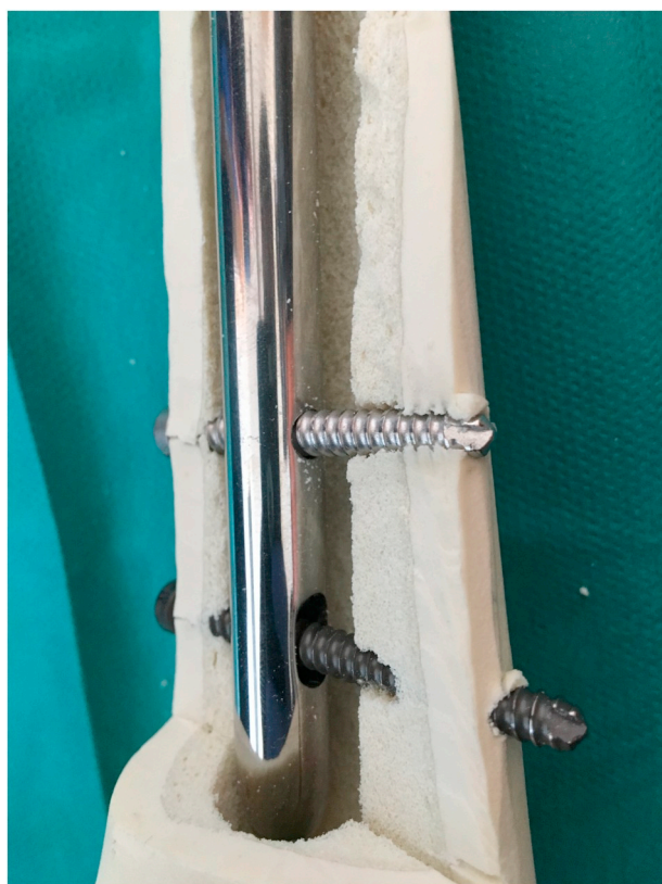
Fig. 5. Distal locking of the long gamma nail. The upper hole is round and tight around the screw, what protects the nail tip from moving from medial to lateral. The lower hole is oblong and unstable.
