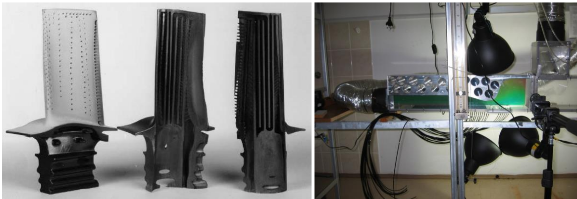
Figure 8. Gas turbine blades with cooling holes (left) and view of test section for model turbine blade cooling (right)
