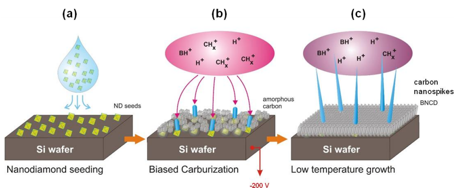
42 Figure 8. Scheme of the growth mechanism of BNCD-CNS hybrids in the H_2/CH_4/B_2H_6/N_2 43 microwave plasma-(a) the nanodiamond seeding on the Si wafer prior to diamond growth, (b) 44 and (c) the sub-sequential steps of nanospike formation of BNCD-CNS hybrids in the microwave 45 plasma. 46 47 48 49
