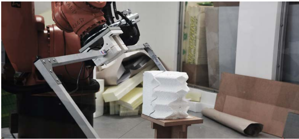
Figure 6: The process of hotwire-cutting with robotic arm.
