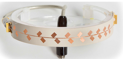
Fig. 12. Measured X-band antenna array on a test fixture: a photograph.
