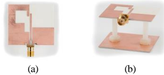
Fig. 7. Photographs of the fabricated antenna prototype: (a) front view, (b) 3D view.
