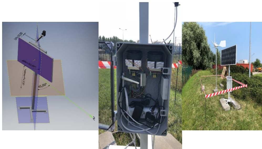
Fig. 4 Block diagram of the system for testing power systems (a), diagram of the mechanical system and view of the test installation (b).
