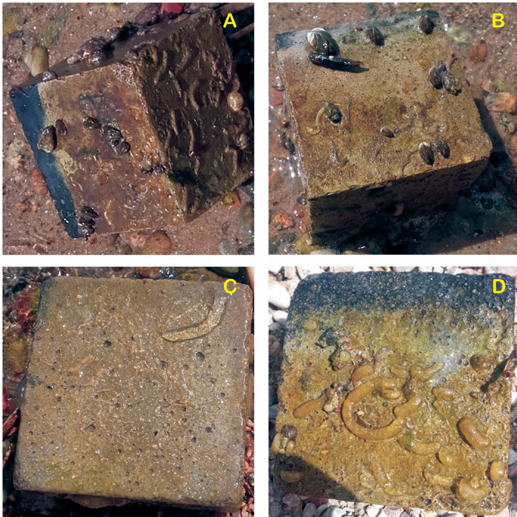
Fig. 7. Image of concrete BP and LB cubes after incubation in a lake for nine months (experiment 2) D. polymorpha growing on the walls: concrete BP (A), and concrete LB (B); packs of mollusc eggs on the side walls: concrete BP (C), concrete LB (D).
