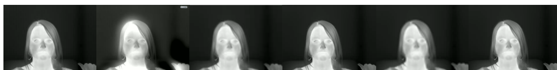
Figure 7. The corresponding frame extracted from the SC3000 8-bit sequences used in the study for respiratory rate evaluation. From the left: original, Eulerian Video Magnification, bicubic interpolation scale 2, super resolved using our model scale 2, bicubic interpolation scale 4, super resolved using our model scale 4.
