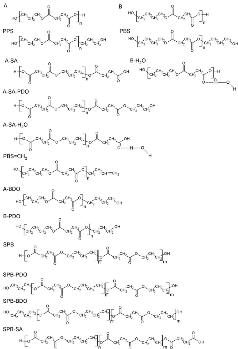
Fig. 6. Probable structure of molecules calculated from MALDI-ToF data.
