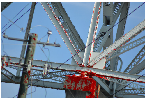
Figure 15. A database of rust colour pixels.
