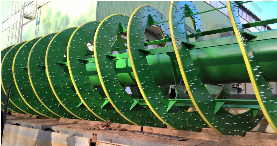
Photo 3. The new spiral of classifier.
