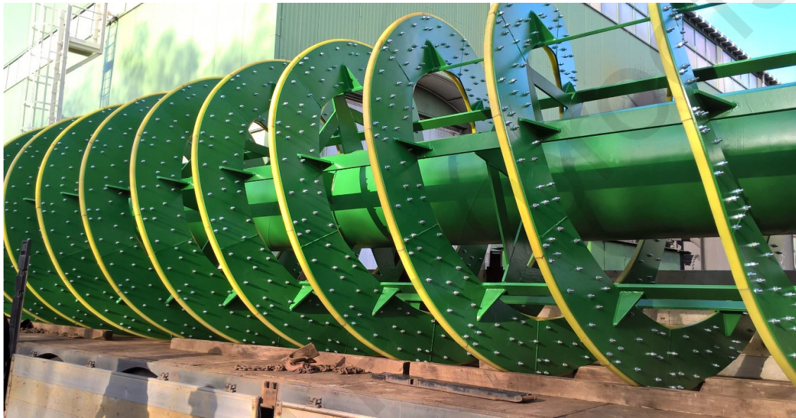
Photo 3. The new spiral of classifier.
