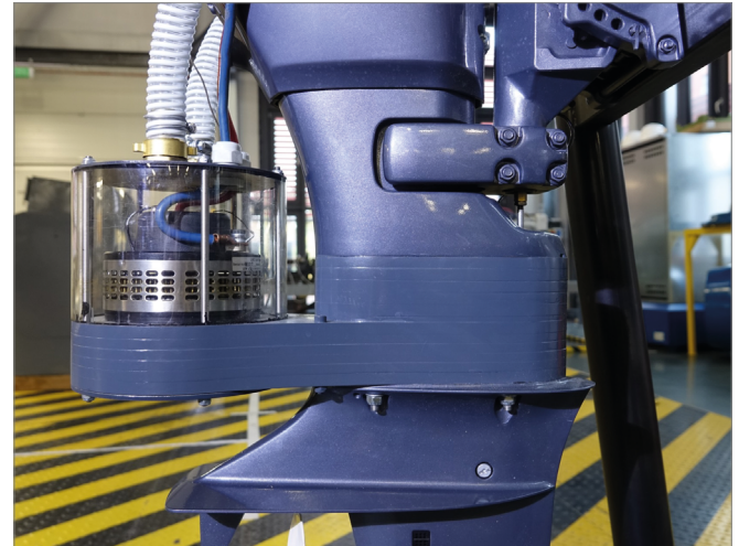
Fig. 4. Electric module installed on the outboard motor base
