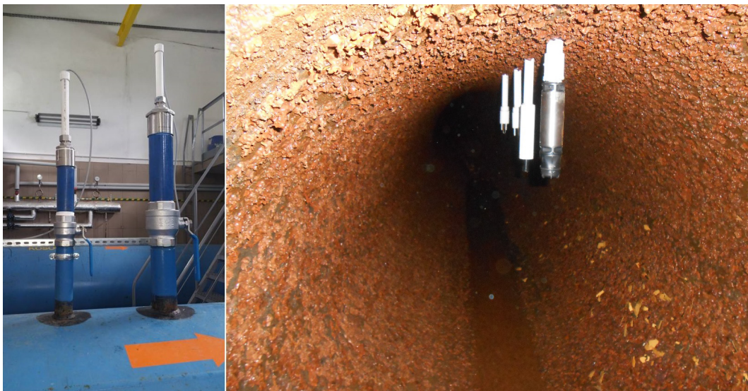
Fig. 2. Assembly of sensors on the left side: view from outside the pipe, on the right side: view from inside the pipe
