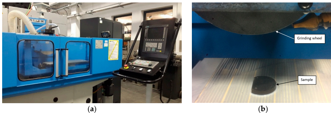
Figure 3. Horizontal-spindle (peripheral) surface grinder SPG 25 × 60: (a) General view, (b) working space with the sample location.
