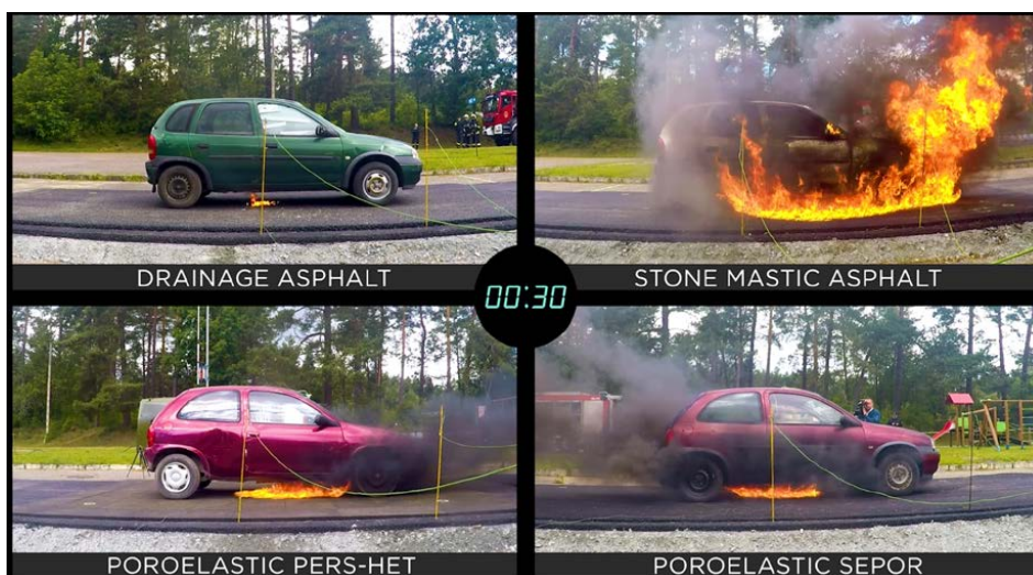
Figure 40. Development of fire 30 s after ignition.
