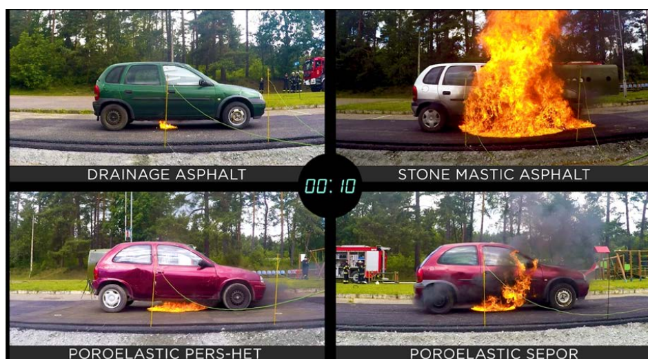
Figure 39. Development of fire 10 s after ignition.
