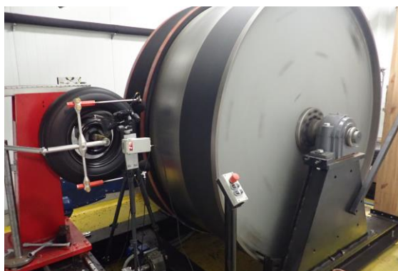
Figure 34. Roadwheel facility at GUT.
