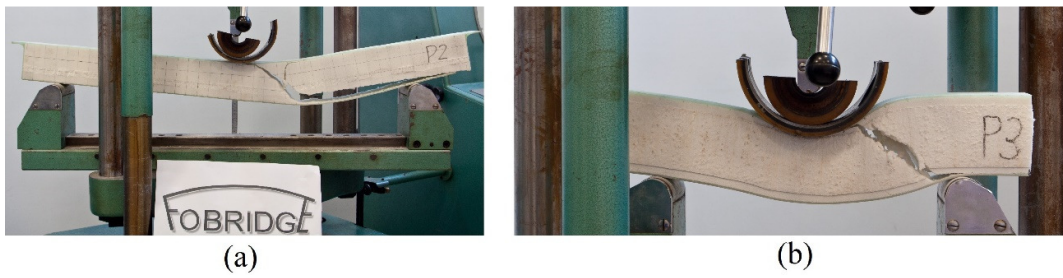
Fig. 1 Preliminary three point bending tests: long (a) and short (b) beams at the moment of failure
