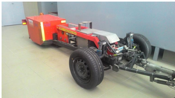
Fig. 2. R2 Mk.2 trailer for measuring the rolling resistance coefficient of tires and pavement [11]
