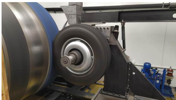
Fig. 3. Roadwheel facility for testing rolling resistance which is part of the Equipment Complex of the Gdańsk University of Technology (own material)
