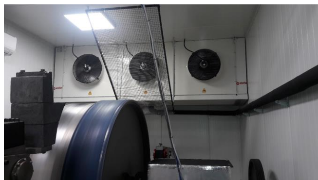
Fig.7. Thermostatic chamber used in the tire testing laboratory of the Gdańsk University of Technology (own material)
