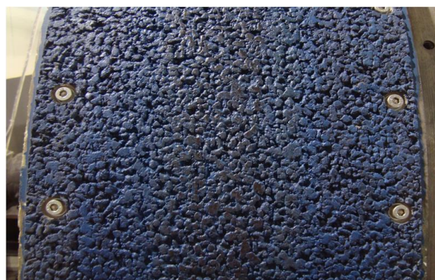
Fig.8. SMA8 surface replica (own material)
