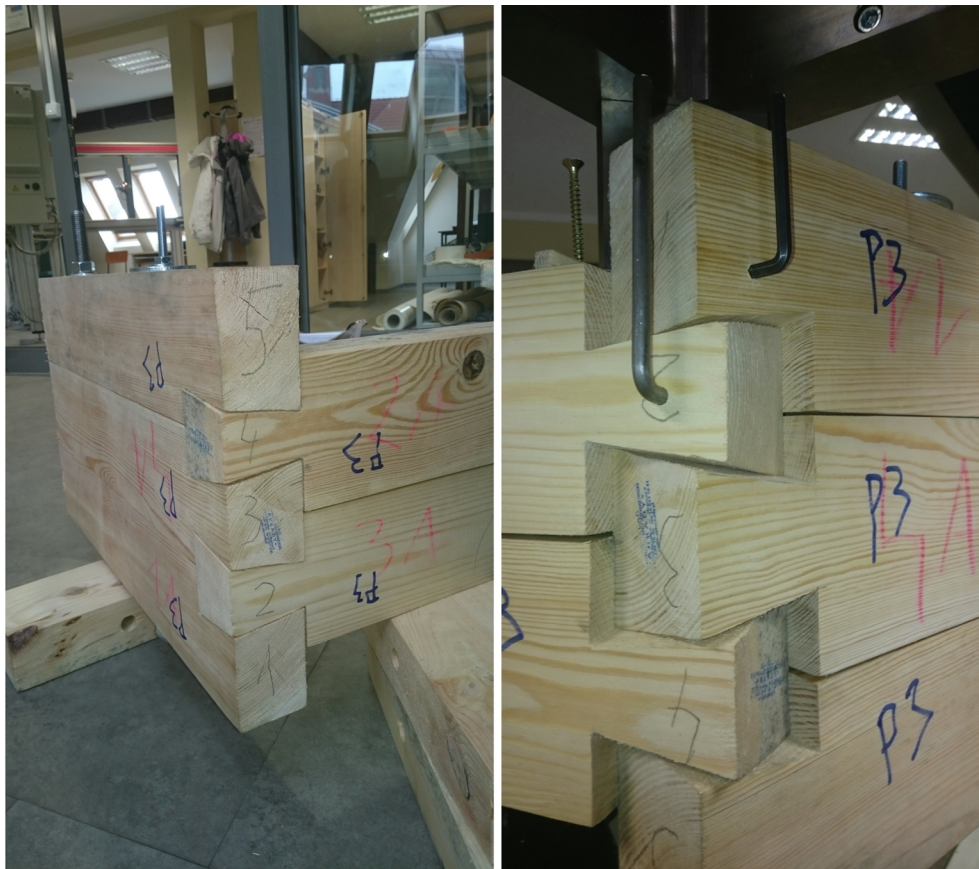
Fig. 6. A dovetail connection before and after the test.
