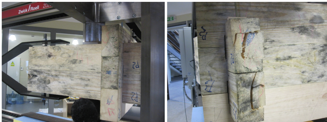
Fig. 7. A saddle-notch connection before and after the test.
