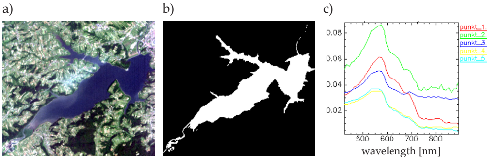
Fig. 2. RGB color composition for the Hyperion image with the marked points of spectrometric measurements (a); mask for the area of the Dobczyce Reservoir (b); spectral curves measured for the waters of the reservoir (c)
