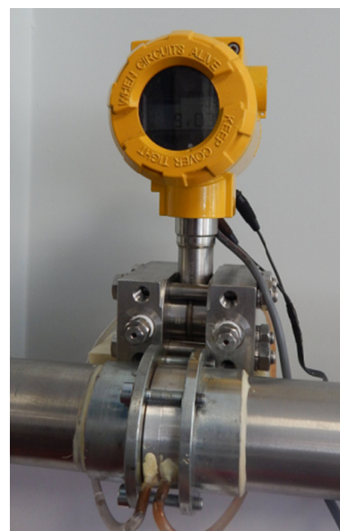
Fig. 10. APR-2000/ALW transducer mounted on the laboratory stand.
