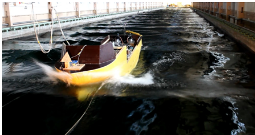
Figure 1. The model tests performed on a free-running reduced-scale model of ship in the deepwater towing tank, located in the Maritime Advanced Research Centre (CTO S.A.) [7].
