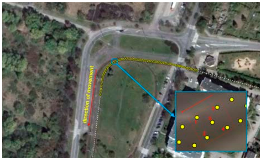
Figure 5. Results of the adjustment of the coordinates of GNSS receiver antennas on a selected section of the tram loop in Gdańsk
