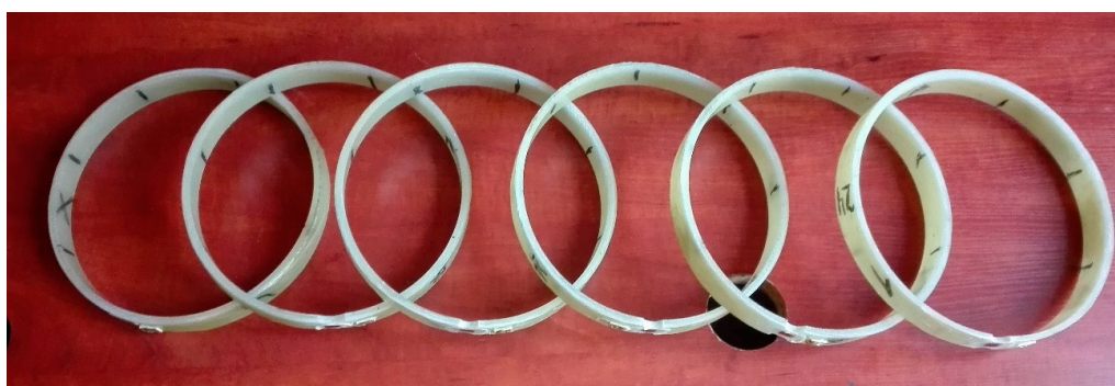
Figure 3. Pipe rims for wall thickness measurements.
