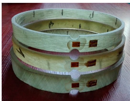
Figure 8. Samples cut from pipes with winding angles of glass fibers \theta = 85^\circ (highest), \theta = 55^\circ (middle) and \theta = 20^\circ (lowest) to test the peripheral tensile strength and modulus of elasticity.
