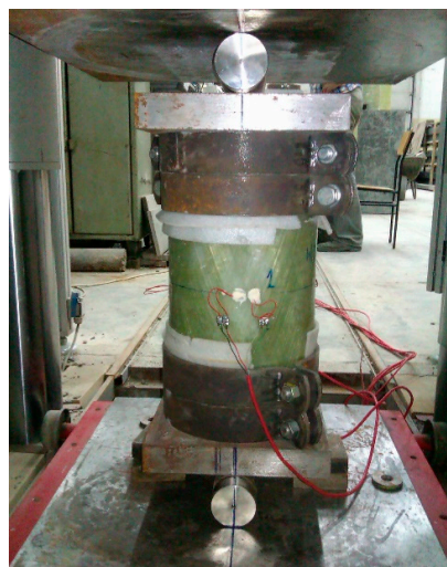
Figure 1. Test element for measuring the mechanical properties of a composite during compression: empty tube with winding angle of 20° on a test stand.
