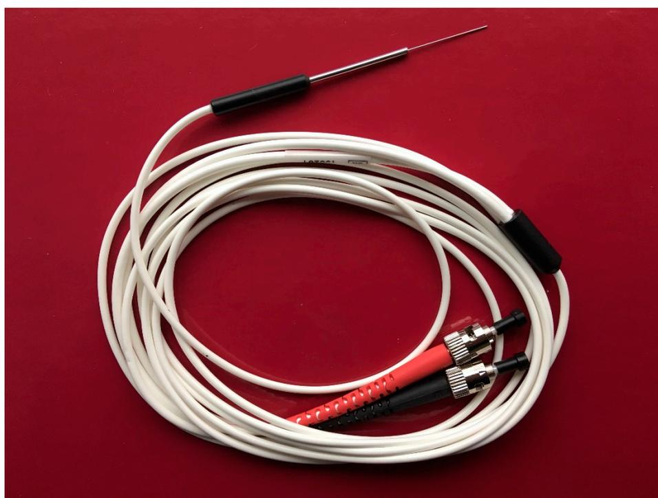
**Figure 1.** Laser Doppler intramuscular fiber-optic perfusion probe.
