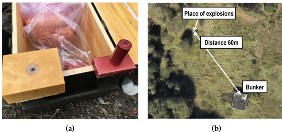
Fig. 1. Photo of explosives samples for tests (a) and MIAT explosive test area: marked distance (60 m) of the bunker from the explosive site (b).
