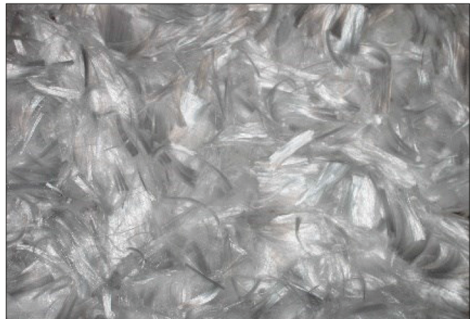
Fig. 3. Polypropylene shrinkage-resistant fibres
