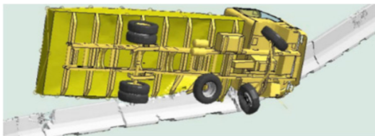
Fig. 6 Vehicle breaks through a barrier during a simulation test
