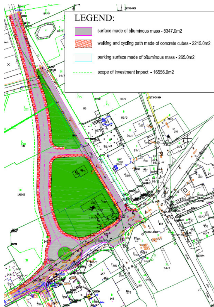
Figure 6. Site plan-proposed solution for the road layout at the intersection—option 1.
