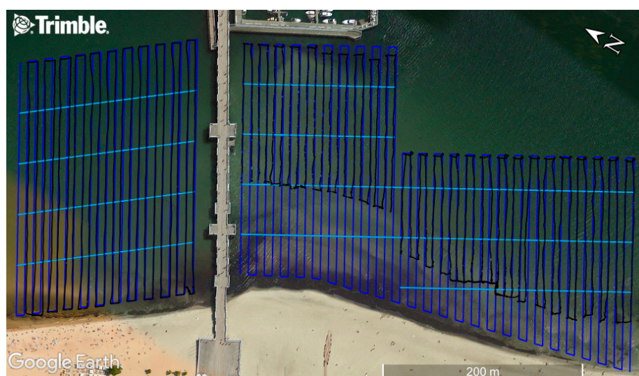
Figure 1. The planned main profiles (blue color) and control profiles (light blue color) along with the plotted trajectory of the Unmanned Surface Vehicle (USV) (black color) during hydrographic surveys of the waterbody adjacent to the Sopot pier.
