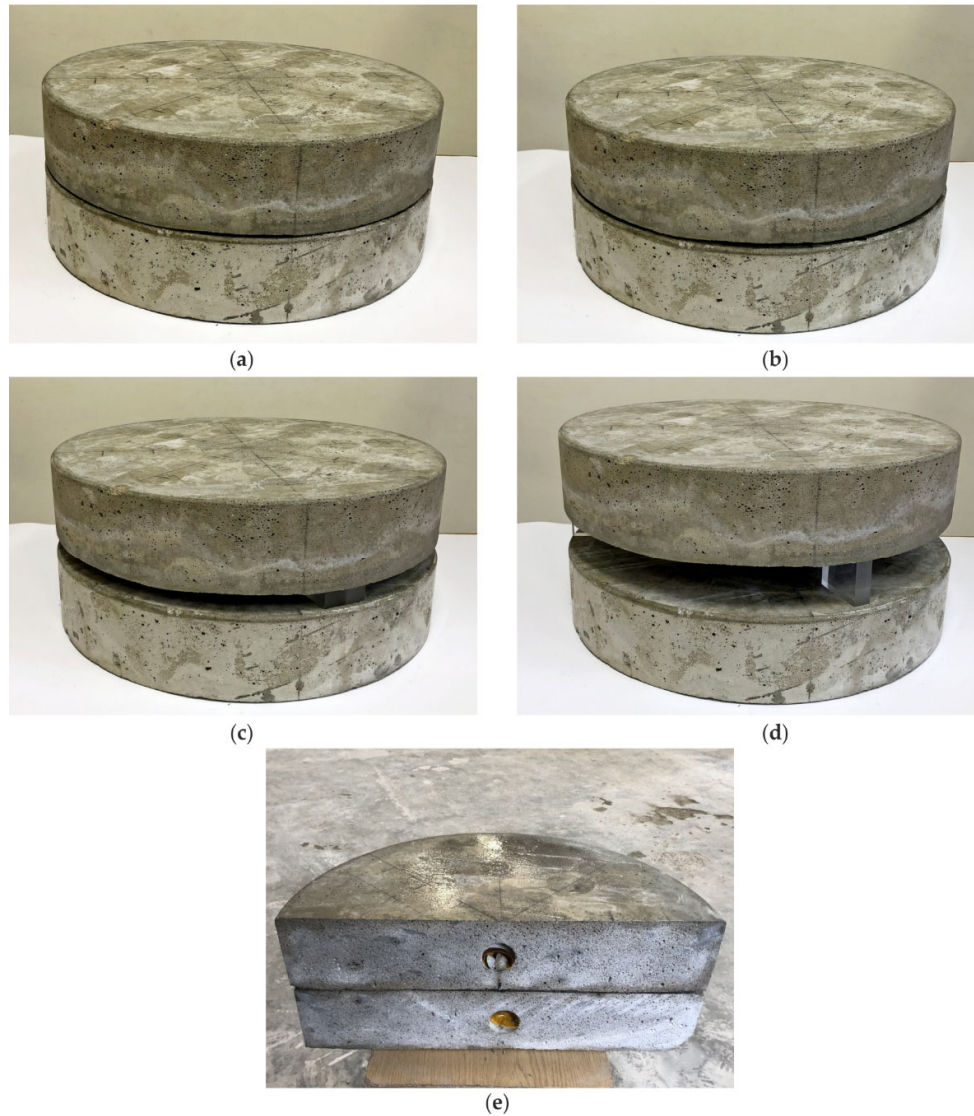
Figure 4. Circular concrete slabs with air gaps of different thickness: (a) 1 mm; (b) 4 mm; (c) 20 mm; (d) 50 mm; and (e) upper plate after cutting.
