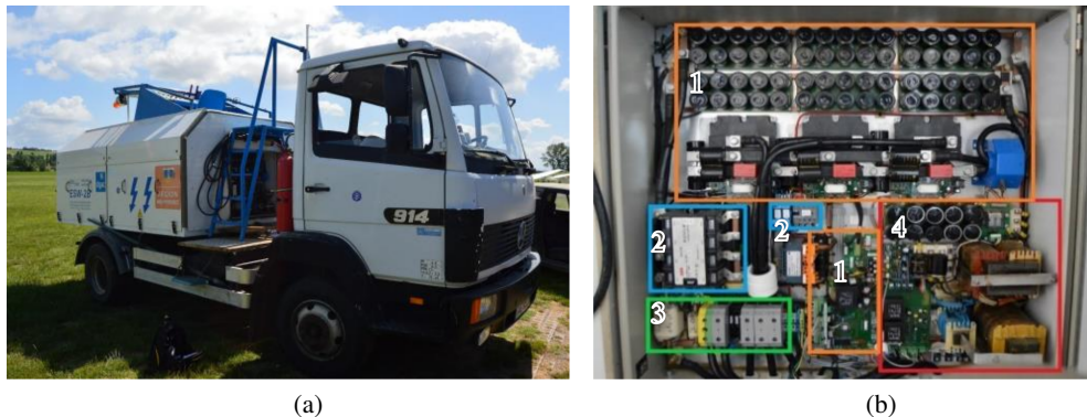
Fig. 1. View of the studied launcher Electronic circuits: (a) Mercedes-Benz model 914; (b) all power electronic components of the launcher (1. inverter with control driver, 2. contractors and relays, 3. fuses, 4. battery charger with driver)
